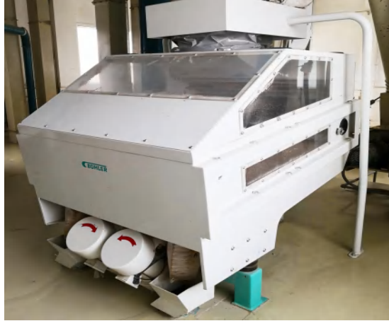
The picture above is a stone removal machine
